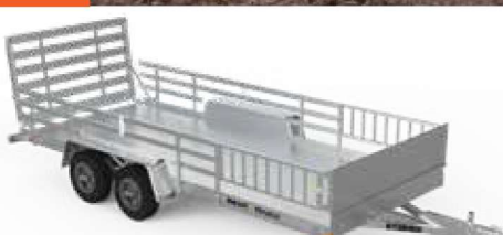
MODEL BTT80192F with rock guard and 3 rail side load open side kit
